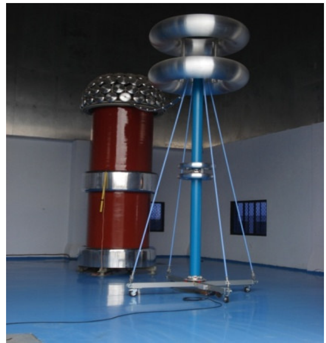
700 kV, High Voltage Transformer
