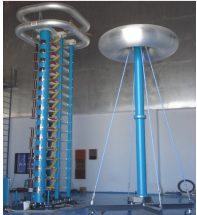
1600 kVp, 80 kJ, Impulse Voltage Generator
