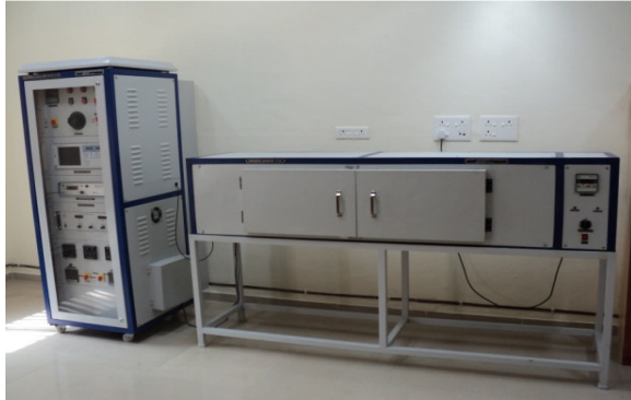
Automated computerized system for T5 lamps testing
