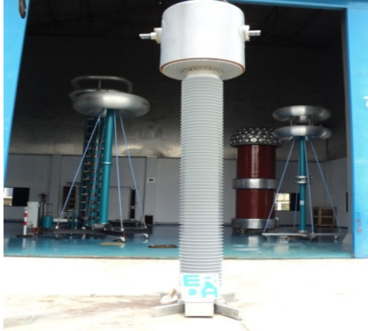
400 kV Current Transformer under High Voltage Test
