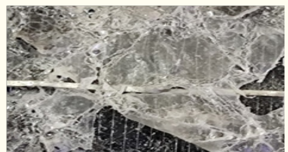
Figure 2.2.1 (a) Photograph of grey colour defect in PV panels striations (a) before removal of glass (b) after removal of glass
